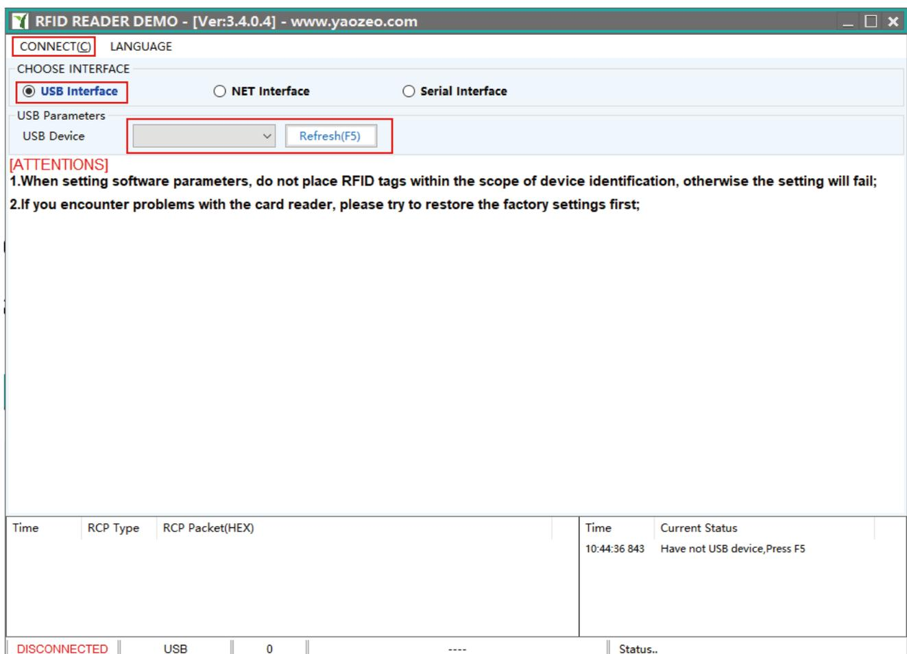
There are three kinds of communication parameter configuration :USB communication -- serial communication -- network port communication.
