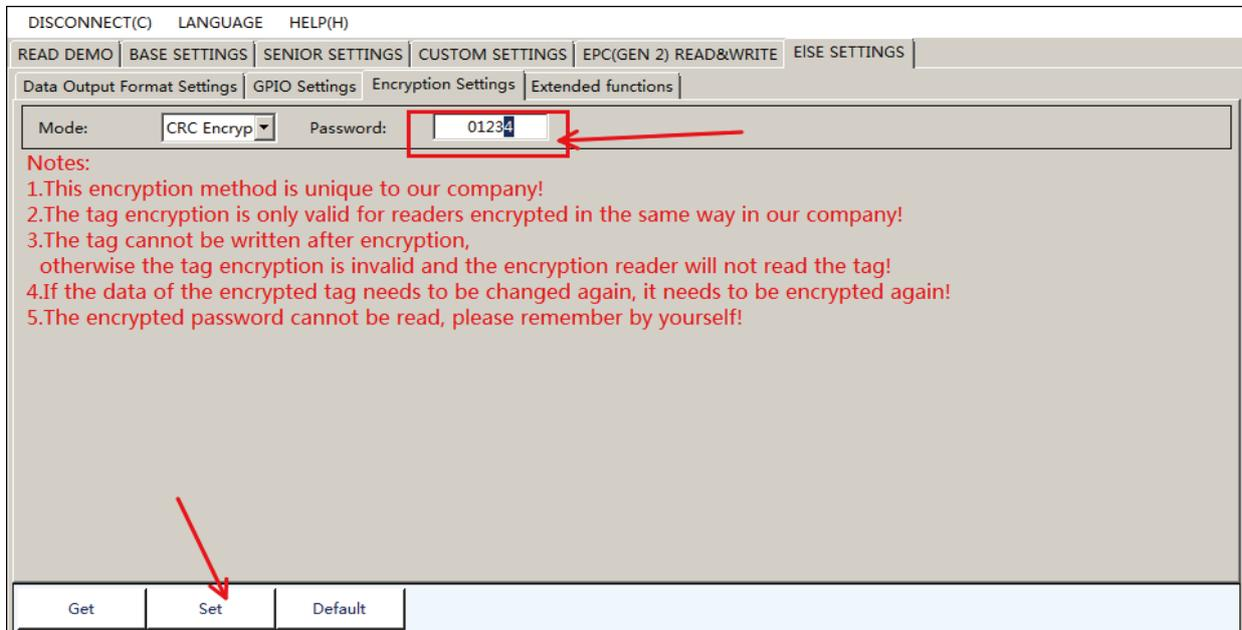
Note 1: The card reader of SG/MG series can only encrypt the card reader. If the tag needs to be encrypted, the card issuer such as DM02 DR201 should be used for encryption. You can refer to another encrypted information.
