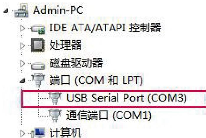
When you unplug the converter, the serial port will disappear. If the computer itself comes with a serial port, it does not need to install the driver, you can directly use.
