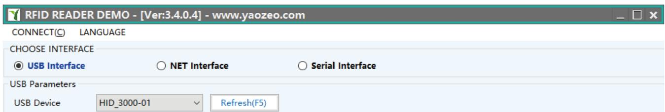
If the USB device is empty, double-check that the USB cable is plugged in, and then press the key
