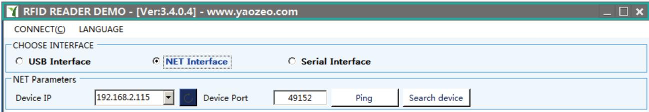
Here, you need to select the correct remote IP address and remote IP port of the device (by default, the computer is a client, the device is a server, and the TCPIP protocol), and click the "Ping" button. If the connection is correct, a success flag will be displayed in the status bar, as shown in the figure:
