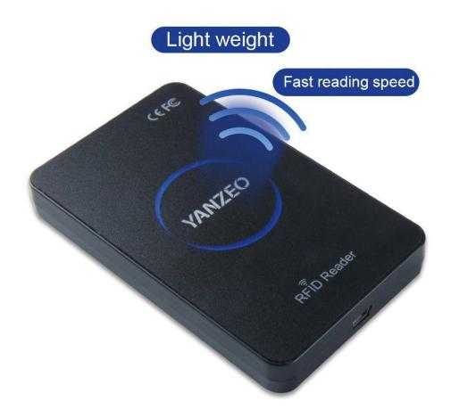
Yanzeo SR360 is a small desktop reader, compatible with ISO 18000-6C standard. Its working frequency is 902MHz~928MHz. It is a small integrated reader for short-distance identification or background card issuer management. It is compact and easy to carry. Suitable for personnel access control, picture document management, and electronic label reading, writing, authorization, formatting and other operations.
