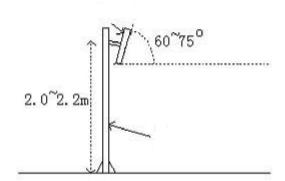
Antenna pitch: refers to the angle between the antenna tilting to the ground and the horizontal line, about 60 to 75 degrees
